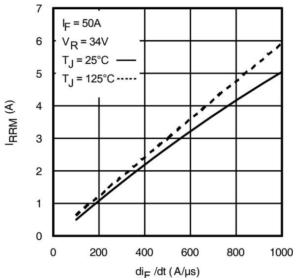
**Fig 20 -** Typical Recovery Current vs.  $di_F/dt$
