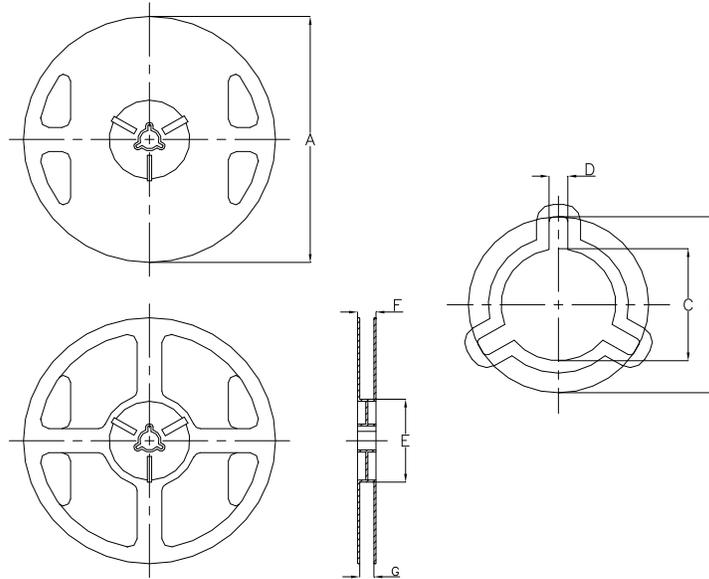
NOTE: Controlling dimensions in mm Std reel quantity is 4000 parts.
