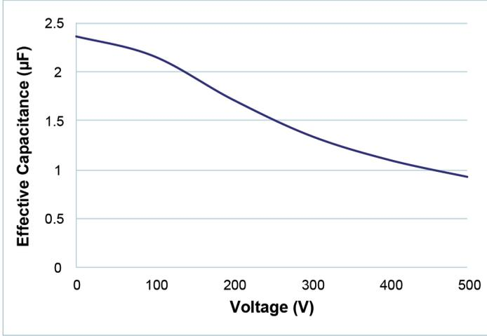
Figure 14 — Effective internal input capacitance vs. applied voltage
