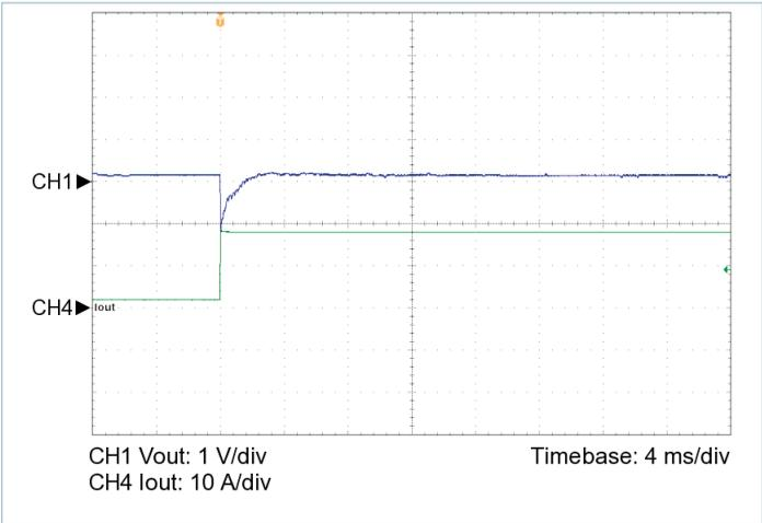
Figure 6 — 10% to 100% load transient response,  $V_{IN} = 270\text{ V}$ , nominal trim,  $C_{OUT\_EXT} = 200\ \mu\text{F}$
