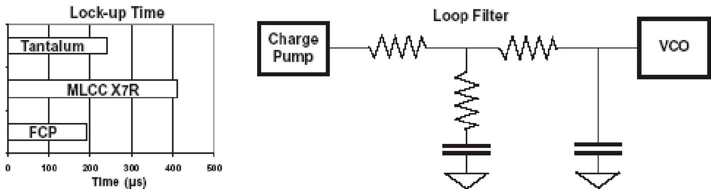
In PLL circuit applications, FCP SMT film capacitor advantages are tight tolerance on the capacitance value, stable capacitance with temperature, faster lock-up times, and no noise due to piezoelectric effects.
