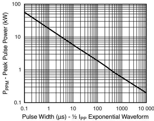
Fig. 1 - Peak Pulse Power Rating Curve
