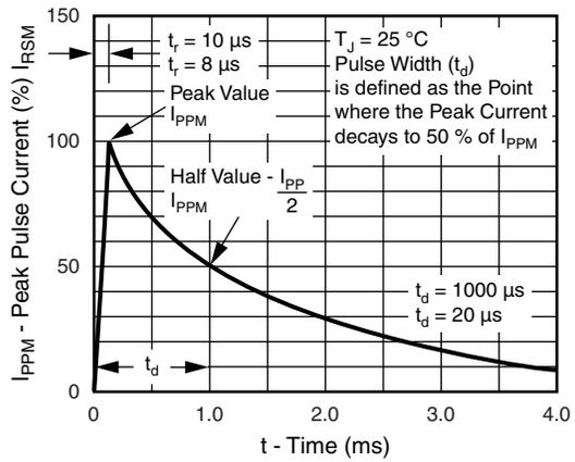
Fig. 3 - Pulse Waveform
