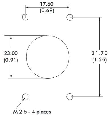
The joystick mounts from beneath the panel and the boot is trapped between the joystick and the panel. No bezel is necessary for this installation, since the panel acts as the bezel. The frame has M2.5 tapped holes and as such M2.5 machine screws are recommended for this mounting.
