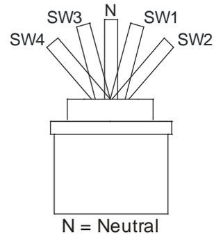
One switch will actuate after 50% of travel, with a further switch at the end of travel, in either direction.
