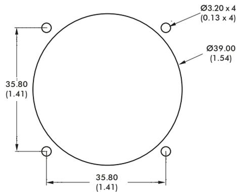
The joystick is dropped into the panel cut-out. For panel thickness of <3mm, M3 x 16 countersunk machine screws are recommended. Please note: Image (left) shows a square bezel, a circular bezel is also available for this option.
