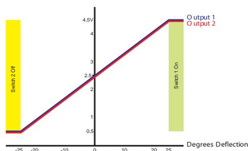
Note: When Dual Output (non-inverted) option is selected the polarity of Switch 2 is inverted
