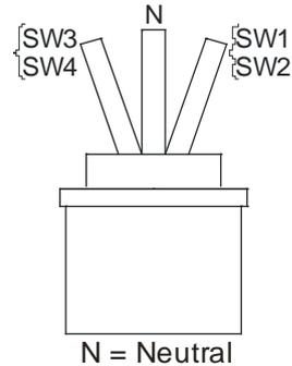
Two switches will actuate as the joystick moves away from center, in either direction.
