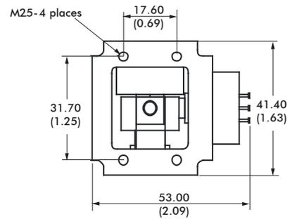
**NOTE:** The dimensions shown are for a generic two axes 4000 Series open body with the E type handle, and a generic two axes 4000 Series closed body also with the two axes E type handle. For specific dimensions of this or any other configuration please refer to Apem.
