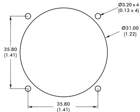
The joystick flange is mounted beneath the panel and the base of the boot must be brought through the panel cut-out and held in place with the circular bezel (option 4). For panel thicknesses of 3mm, M3 x 16 countersunk machine screws are recommended.
