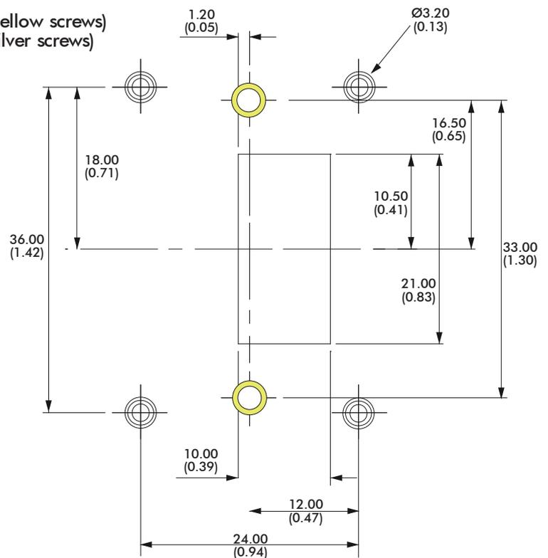
The Paddle is fitted with M3 bushes in all six positions, as standard.
