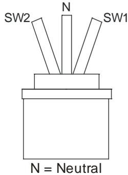
One switch will actuate as the joystick moves away from center in either direction.
