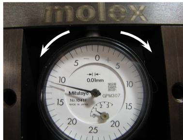
Shut height is less than 135.8mm
