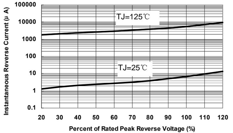
Fig.2-Typical Reverse Characteristics
