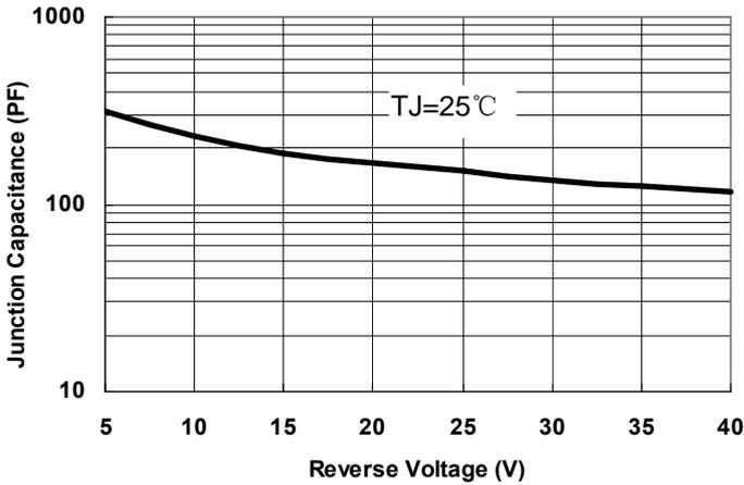
Fig.1-Typical Junction Capacitance
