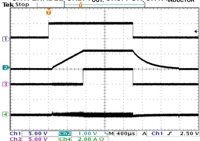
**Power Up/Down at 0.6 Ω Load ( $V_{IN} = 5\text{ V}$ ,  $V_{OUT} = 1.2\text{ V}$ )**
