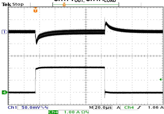
**Transient Response at  $V_{IN} = 5\text{ V}$**
