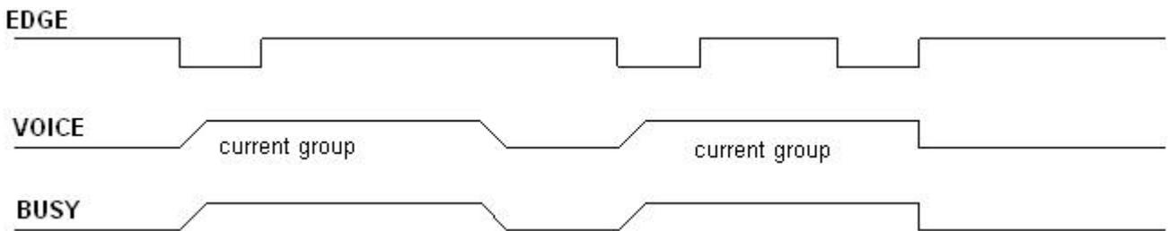
Remark: Edge trigger. When I/O test falling edge( such as this I/O short touch GND) ,the voice will be triggered. After play finished, will stop . During the playing , the next falling edge will stop the voice ,other falling edge will make it play again.
