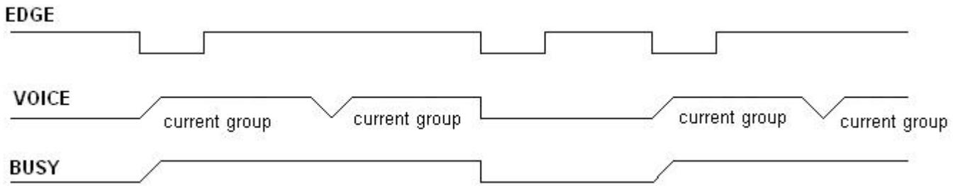
Remark: Edge trigger. When I/O test falling edge( such as this I/O short touch GND) ,the voice will be triggered. After play finished, will cycle play. During the playing , the next falling edge will stop the voice ,other falling edge will make it play again
