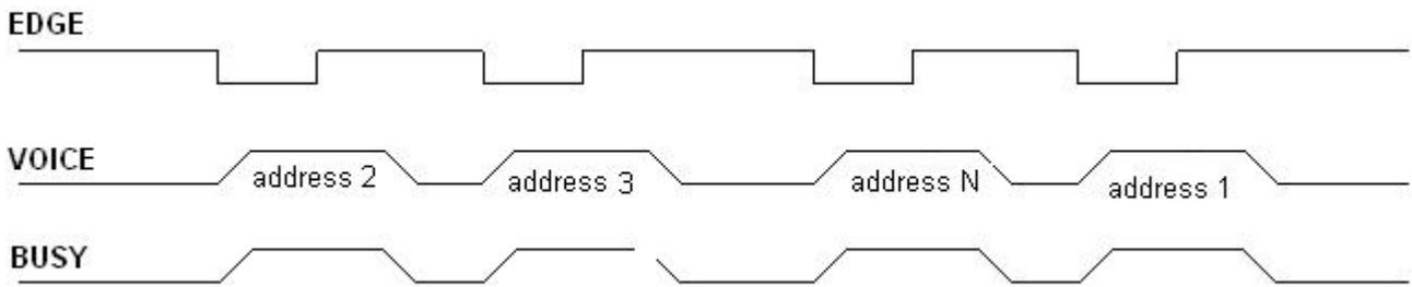
Remark: Edge trigger. One key trigger one group of voice. A negative edge trigger a group of voice, next negative edge trigger next group of voice, after finish last group loop to first group.
