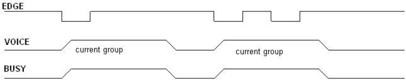
Remark: Edge trigger. When I/O test falling edge( such as this I/O short touch GND) ,the voice will be triggered. During the playing , the next falling edge will not interrupt the voice,after voice play finished,falling edge will make it replay .
