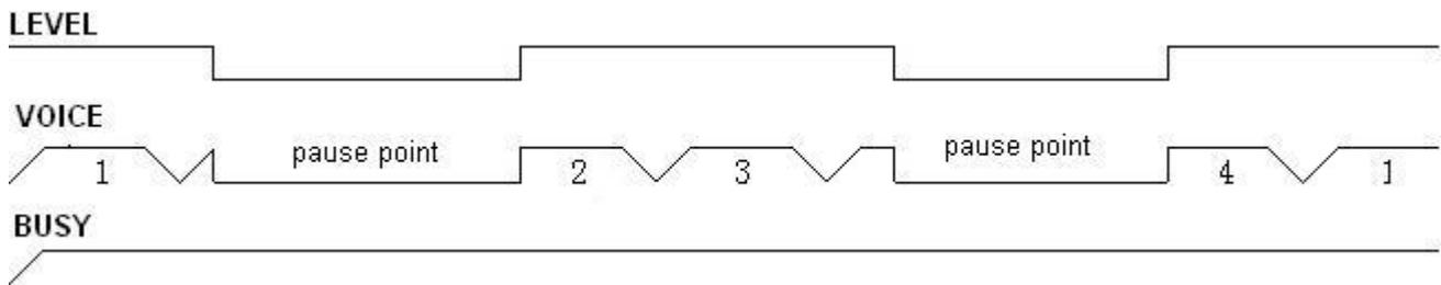
Negative level trigger. Power on , it will play automatically, negative level trigger P05 to pause , next trigger to play from the pause point. After voices play finished, it will loop .
