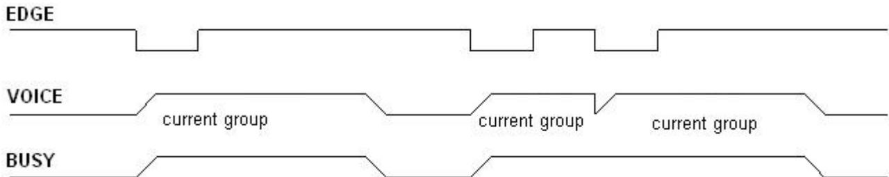
Remark: Edge trigger. When I/O test falling edge( such as this I/O short touch GND) ,the voice will be triggered. During the playing , the next falling edge will interrupt the voice and replay from beginning.
