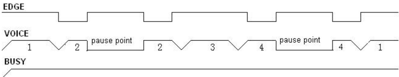
Negative edge trigger. Power on , it will play automatically, negative edge trigger P04 to pause , next trigger to play from the pause point. After voices play finished, it will loop .
