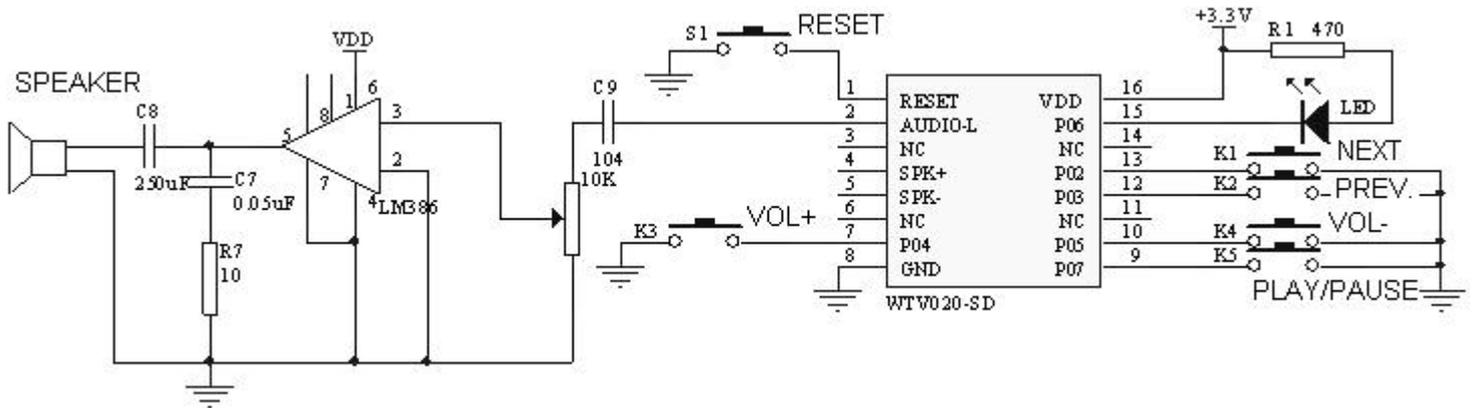
WTV020-SD-16P DAC output, "Audio L" and module GND to amplifier. WTV020-SD-20S DAC output, "SPK+" and module GND to amplifier.
