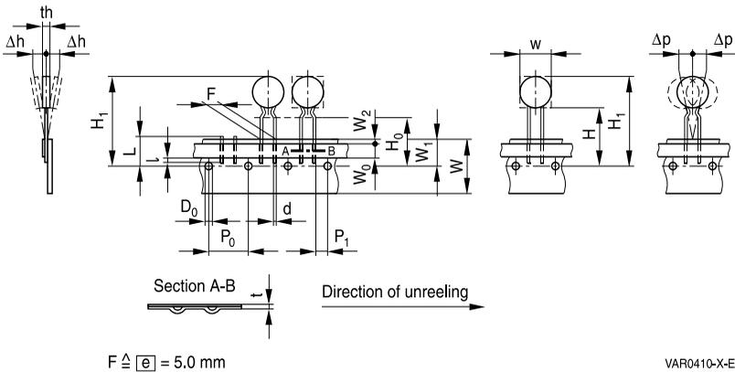
**2.2 Taping based on IEC 60286-2 for lead spacing 7.5 and 10 mm**
