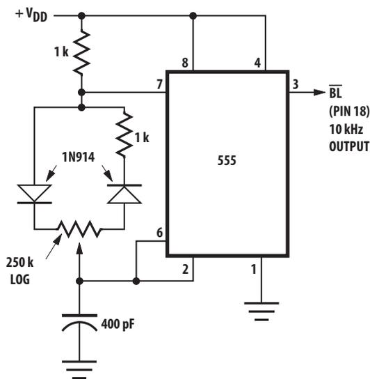
Figure 3 shows a circuit designed to dim the display from 98% to 2% by pulse width modulating the  $\overline{BL}$  input. A logarithmic or a linear potentiometer may be used to adjust the display intensity. However, a logarithmic potentiometer matches the response of the human eye and therefore provides better resolution at low intensities. The circuit frequency should be designed to operate at 10 kHz or higher. Lower frequencies may cause the display to flicker.
