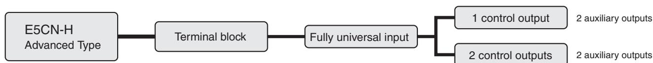
**Note:** Models with one control output and models with two control outputs can be used for heating/cooling control.
