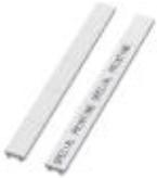
Contactor marker – zack marker strip, Can be ordered: Strip, white, Labeled according to customer specifications, Mounting type: Snap into flat marker groove, Lettering field: 17.5 x 8 mm
