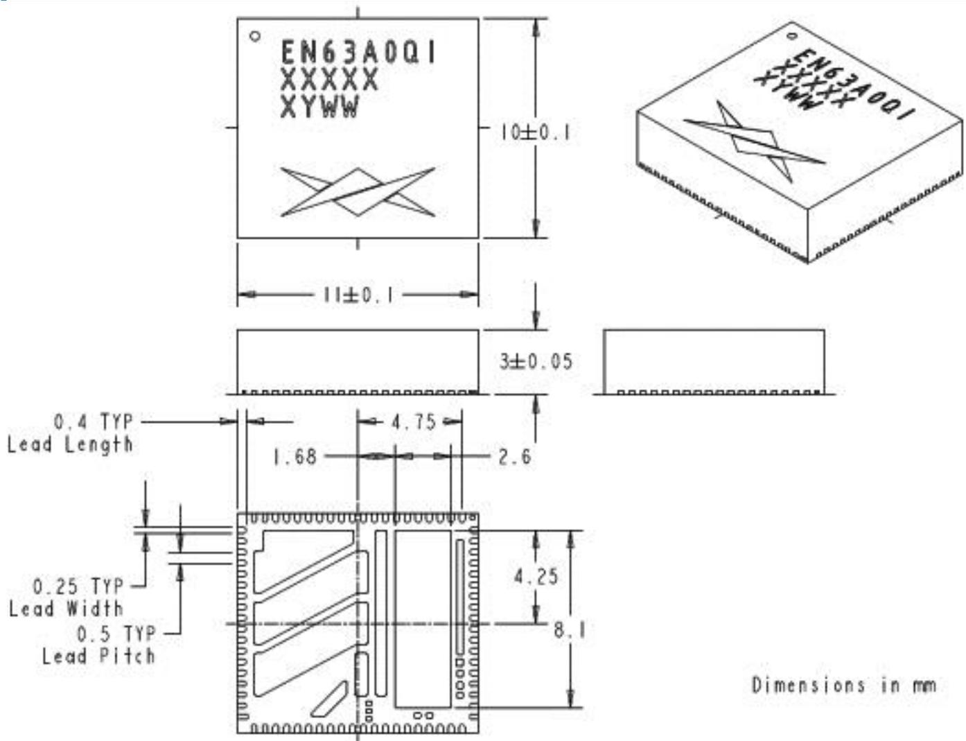
Figure 13. EN63A0QI Package Dimensions (Bottom View)
