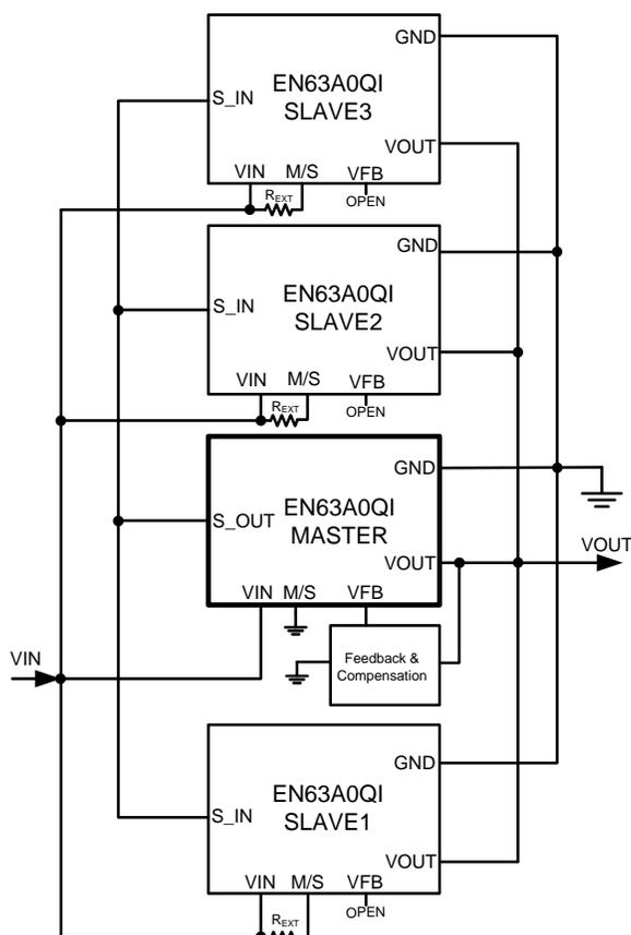
**Figure 5.** Master/Slave Parallel Operation Diagram
