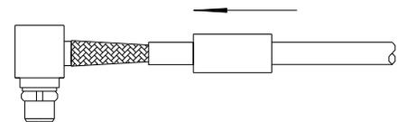
7. CRIMP OUTER FERRULE WITH APPROPRIATE CRIMP TOOL.
