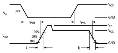
Figure 1. Switching Waveforms
