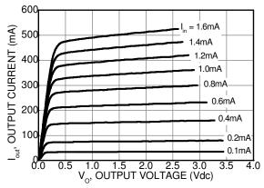
Figure 5. Transistor Output V-I Characteristic
