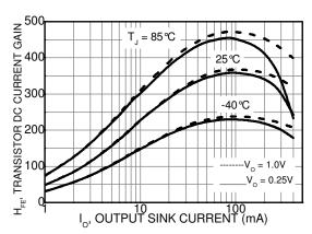
Figure 2. Transistor DC Current Gain
