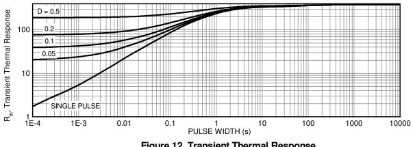
Figure 12. Transient Thermal Response
