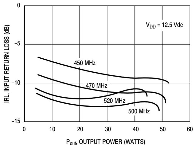
Figure 12. Input Return Loss versus Output Power
