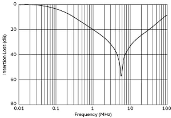
Differential Mode Insertion Loss (Typ.)
