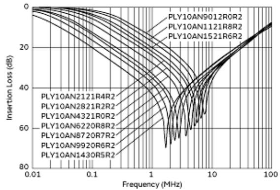
Differential Mode Insertion Loss-Frequency Characteristics
