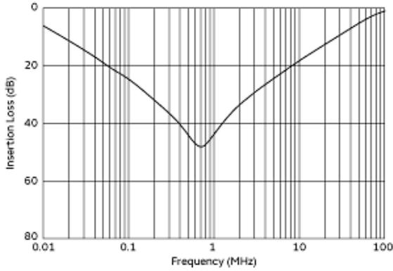
Common Mode Insertion Loss (Typ.)
