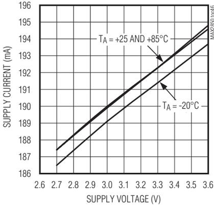
**QUAD Tx SUPPLY CURRENT vs. SUPPLY VOLTAGE**
