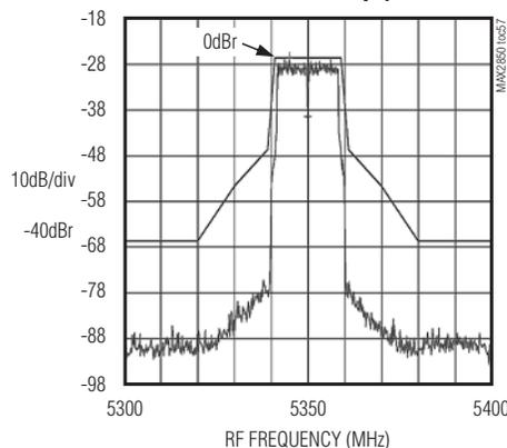
**Tx CARRIER LEAKAGE vs. RF FREQUENCY**
