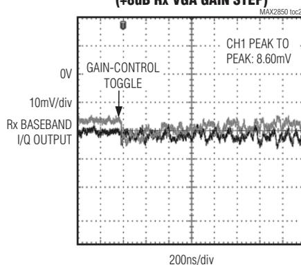
**Rx DC OFFSET SETTLING RESPONSE (+16dB Rx VGA GAIN STEP)**
