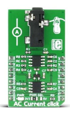
**AC Current click** can measure alternating currents **up to 30A** and it features the MCP3201 ADC (analog to digital) converter and the MCP607 CMOS Op Amp, both from Microchip. The click is designed to run on either 3.3V or 5V power supply. It communicates with the target MCU over an SPI interface, and the AN pin on the mikroBUS<sup>TM</sup> line.
