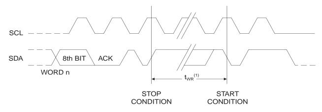
Note: 1. The write cycle time t<sub>WR</sub> is the time from a valid stop condition of a write sequence to the end of the interval clear/write cycle.
