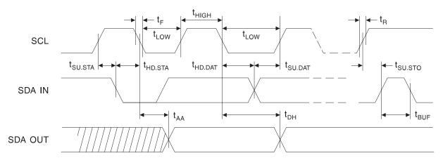
Write Cycle Timing (SCL: Serial Clock, SDA: Serial Data I/O)
