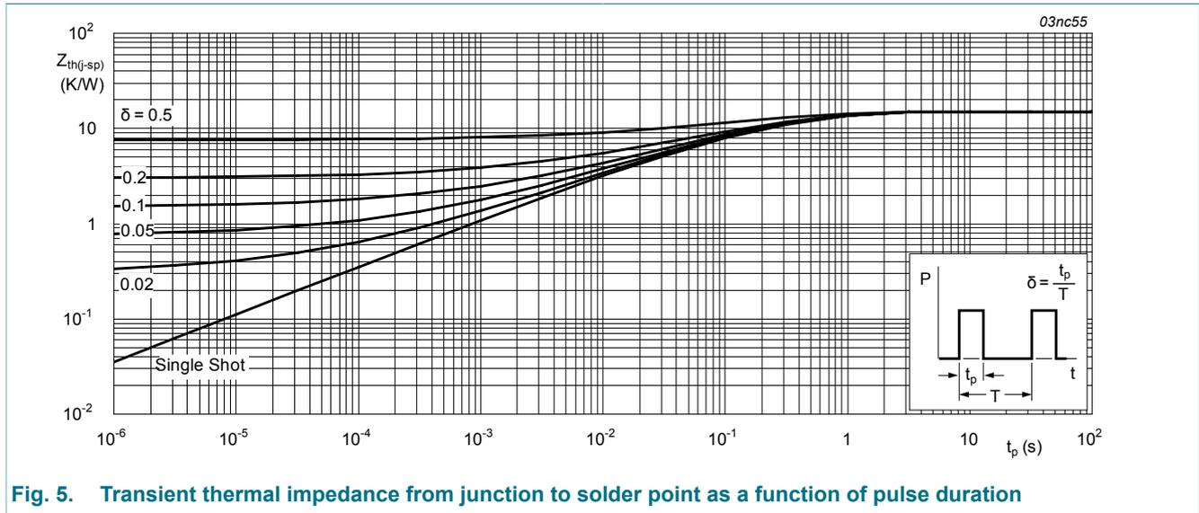
Fig. 5. Transient thermal impedance from junction to solder point as a function of pulse duration
