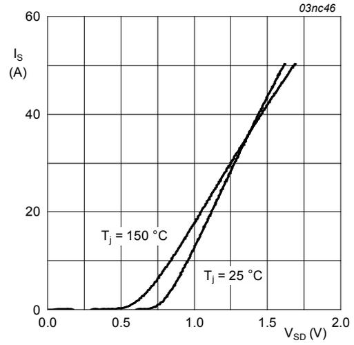
**Fig. 17. Reverse diode current as a function of reverse diode voltage; typical value**
