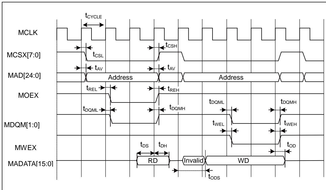
**13.5.7.5 Multiplexed Bus Access Asynchronous SRAM Mode**
