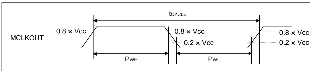
13.5.7.2 External bus signal input/output characteristics
