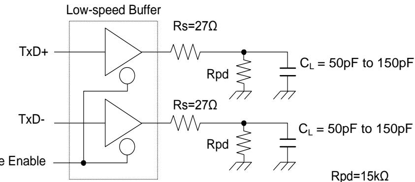
**13.7.2 Low-Speed Load (Downstream Port Load) - Reference 2**
