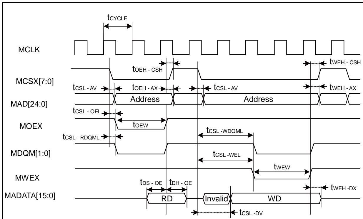
**13.5.7.4 Separate Bus Access Synchronous SRAM Mode**
