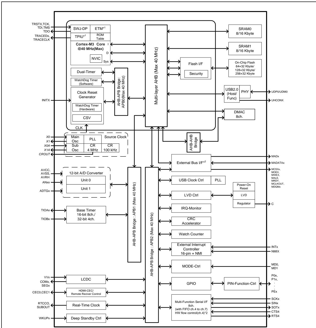
\*1:For the MB9AFB41LB/MB, MB9AFB42LB/MB, and MB9AFB44LB/MB, ETM is not available.
