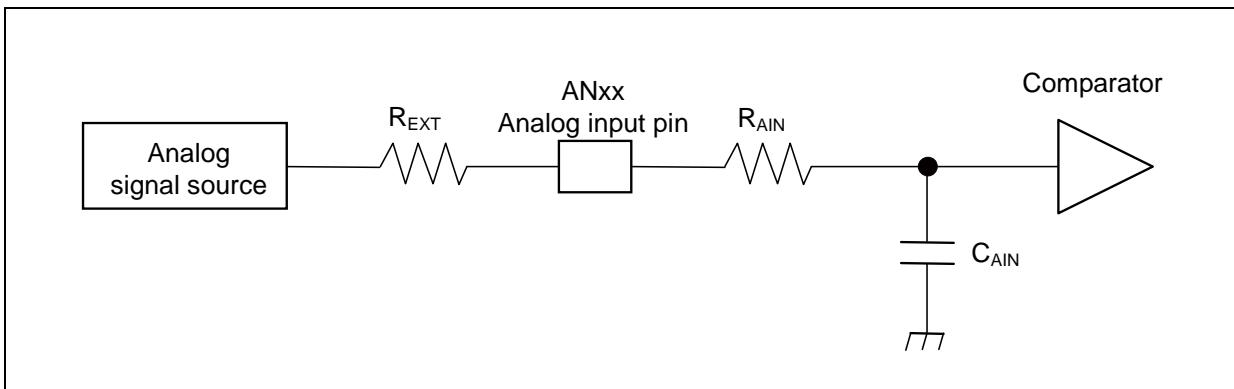
$$(\text{Equation 1}) \quad t_s \geq (R_{AIN} + R_{EXT}) \times C_{AIN} \times 9$$
