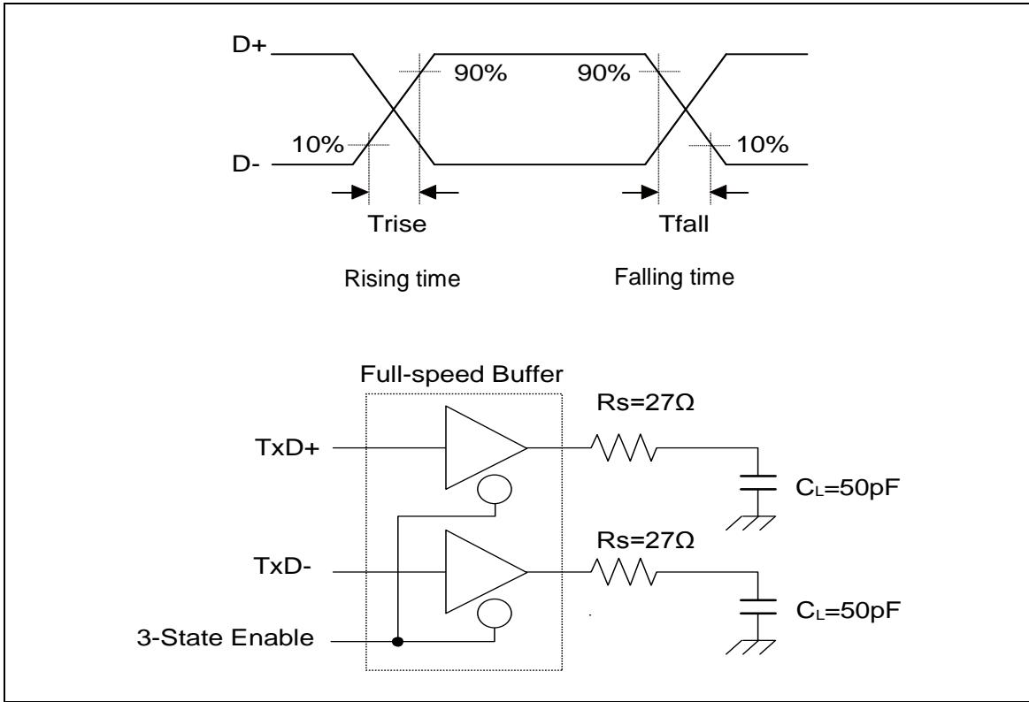
[6]: USB Full-speed connection is performed via twist pair cable shield with  $90\Omega \pm 15\%$  characteristic impedance (Differential Mode). USB standard defines that output impedance of USB driver must be in range from  $28\Omega$  to  $44\Omega$ . So, discrete series resistor ( $R_s$ ) addition is defined in order to satisfy the above definition and keep balance. When using this USB I/O, use it with  $25\Omega$  to  $30\Omega$  (recommendation value  $27\Omega$ ) Series resistor  $R_s$ .
