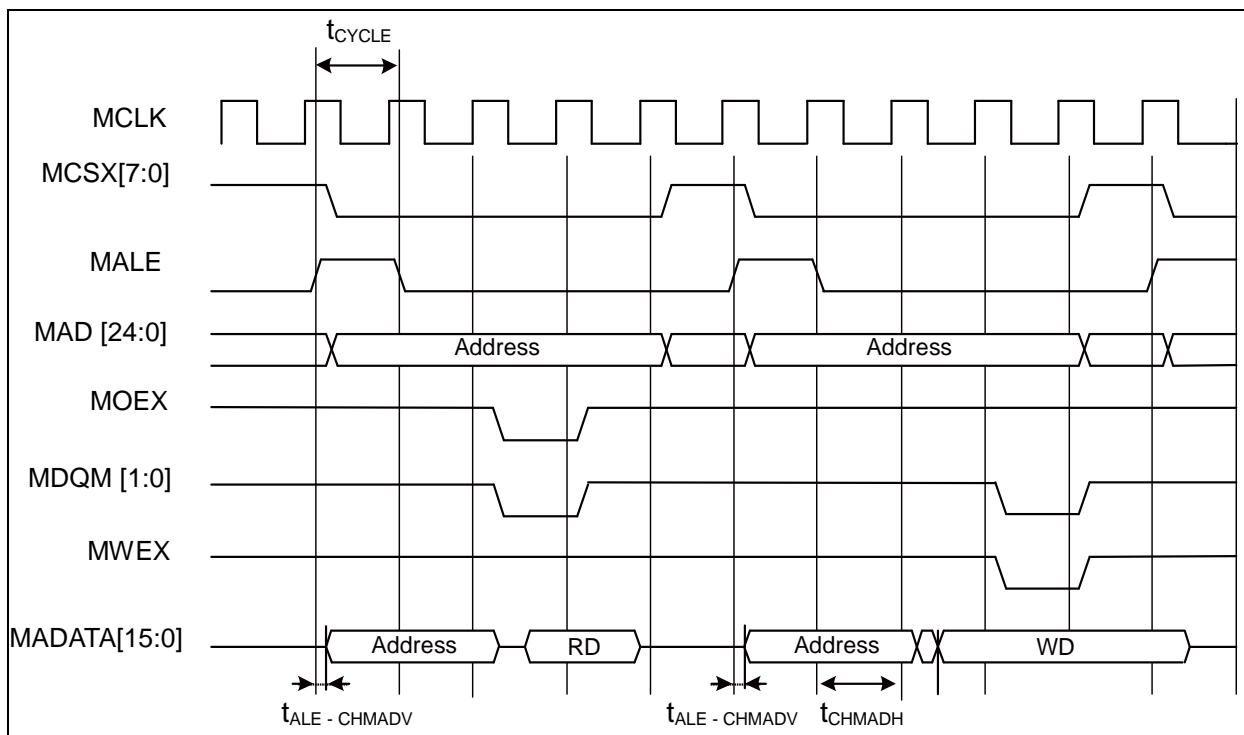
**13.5.7.6 Multiplexed Bus Access Synchronous SRAM Mode**
