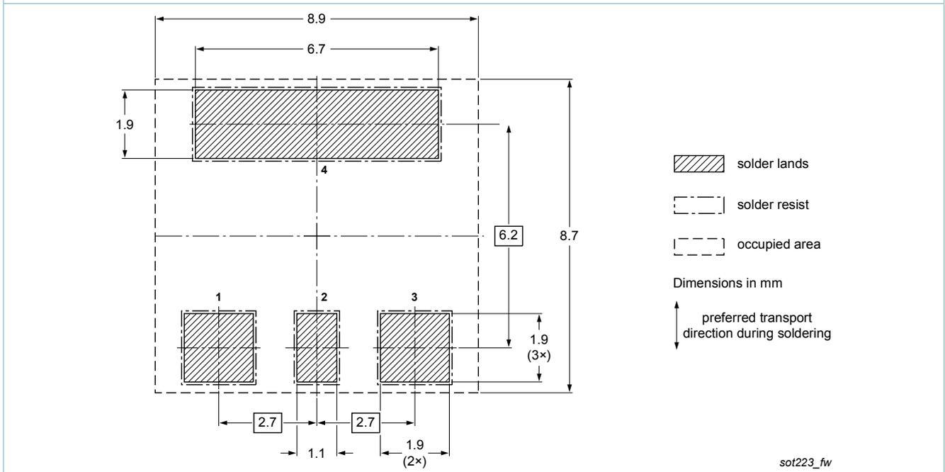
Fig. 13. Wave soldering footprint for SC-73 (SOT223)
