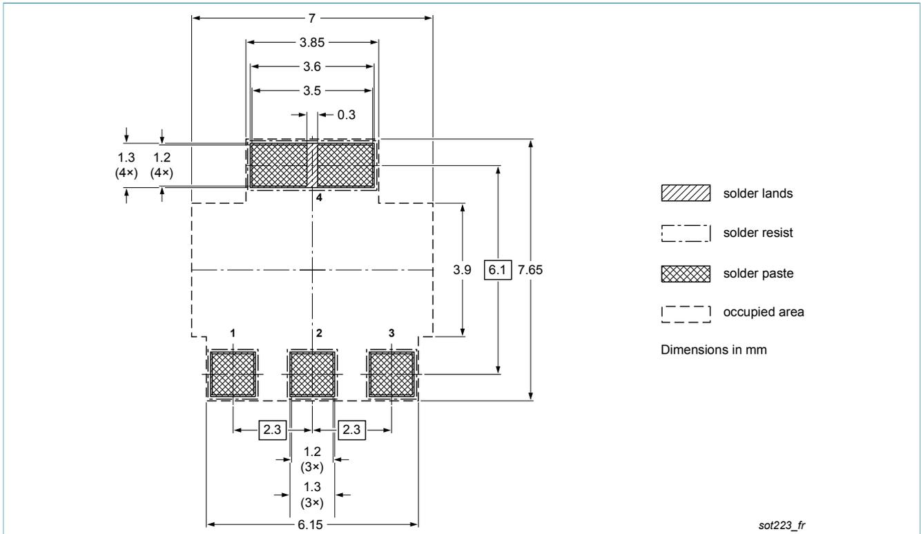
Fig. 12. Reflow soldering footprint for SC-73 (SOT223)
