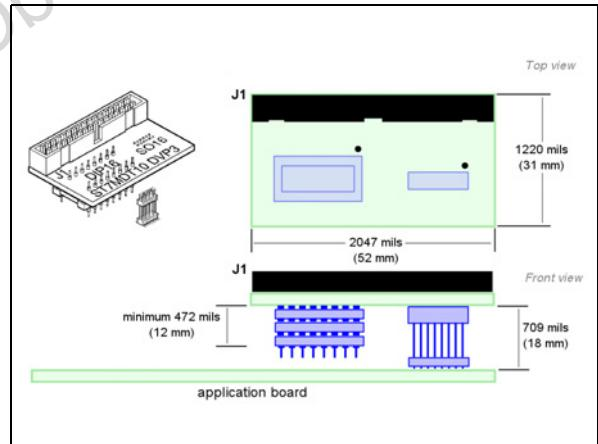
Figure 2. DIP16 application board connection
