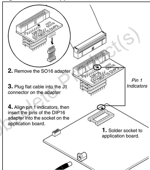
Figure 3. SO16 application board connection
