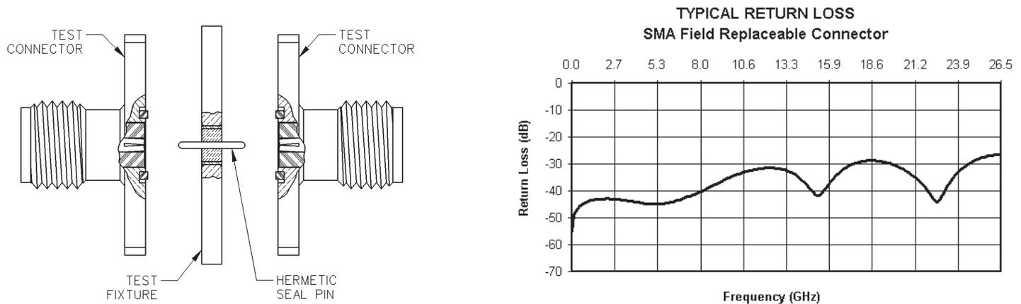
Although Johnson Components™ does not publish a VSWR specification for field replaceable connectors, typical connector VSWR can be expected to be less than  $1.1 + .01f$  (f in GHz). A VSWR specification is not stated because an industry standard method for testing field replaceable connectors does not exist. The actual performance of the connector is dependent upon the application for the following reasons:
