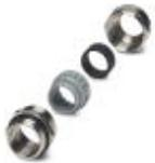
Metal screw connection up to 5 bar, thread length: 8 mm, cable diameter: 14 - 21 mm, WAF 34, screw connection: M32
