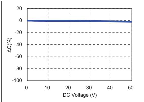
4) Bias TCC characteristics (Agilent 4284A, 1kHz, 1.0Vrms, 25Vdc)
