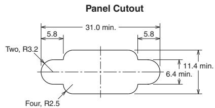
Note: The mounting hole and panel cutout dimensions are the same for the Sockets and Plugs.
