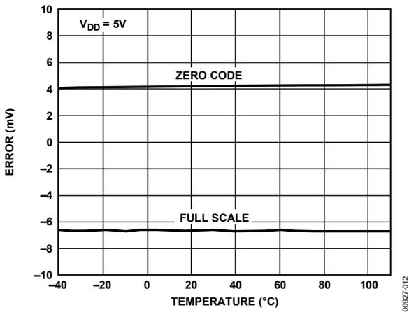
Figure 12. Zero-Code Error and Full-Scale Error vs. Temperature
