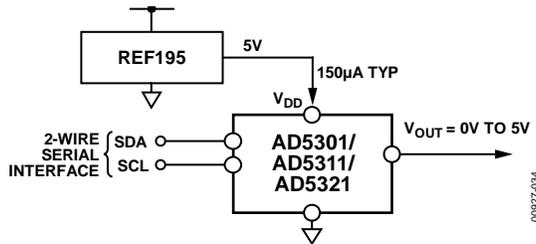
Figure 36. REF195 as Power Supply to AD5301/AD5311/AD5321
