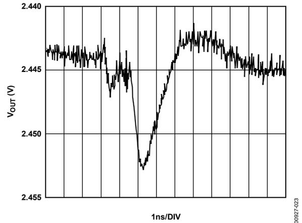
Figure 23. Digital Feedthrough
