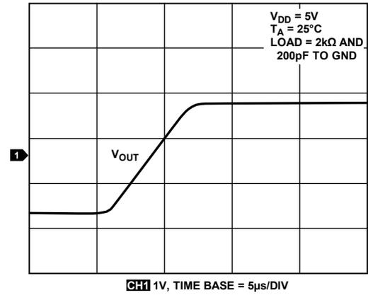
Figure 19. Half-Scale Settling (1/4 to 3/4 Scale Code Charge)
