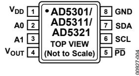
Figure 3. 8-Lead MSOP (RM-8) Pin Configuration
