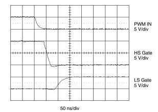
Figure 5. PWM Signal vs. HS Gate and LS Gate (Falling)
