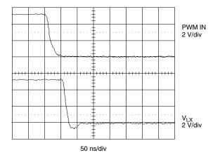
Figure 3. PWM Signal vs. LX (Falling)
