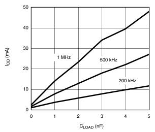
I<sub>DD</sub> vs. C<sub>LOAD</sub> vs. Frequency
