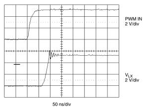
Figure 2. PWM Signal vs. LX (Rising)
