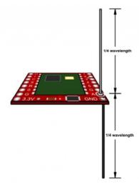
Keep both wires straight, in free air, and away from large metal objects if possible.
