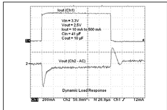
**FIGURE 2-30:** Dynamic Load Response (10 mA to 500 mA).
