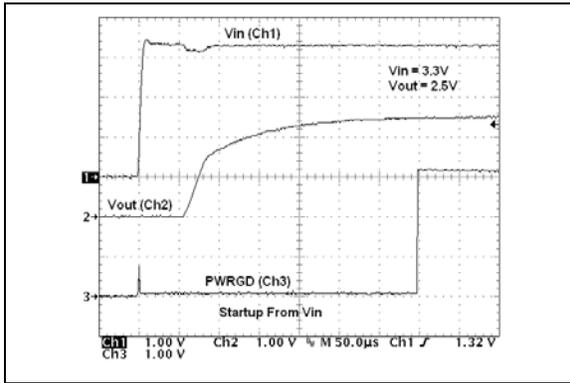
**FIGURE 2-25:** 2.5V (Adj.) Startup from  $V_{IN}$ .
