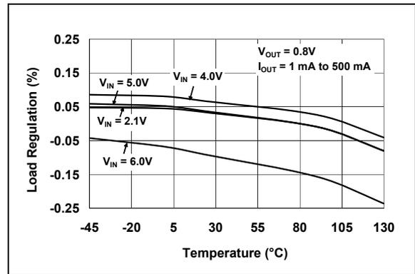
**FIGURE 2-17:** Load Regulation vs. Temperature ( $V_{OUT} < 2.5\text{V}$  Fixed).
