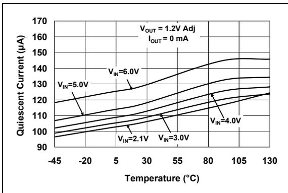
**FIGURE 2-3:** Quiescent Current vs. Junction Temperature (Adjustable Version).
