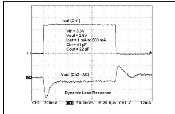
**FIGURE 2-29:** Dynamic Load Response (1 mA to 500 mA).
