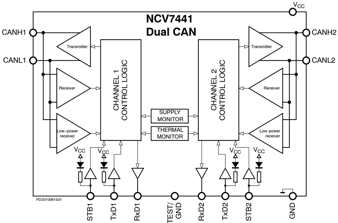
Figure 1. NCV7441 Dual CAN: Block Diagram
