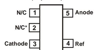
\*must be left floating or connected to pin 5
