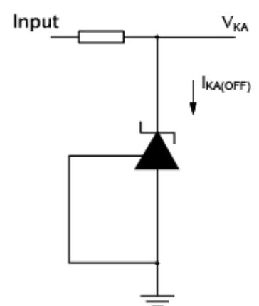
Figure 3. Test circuit for off state current
