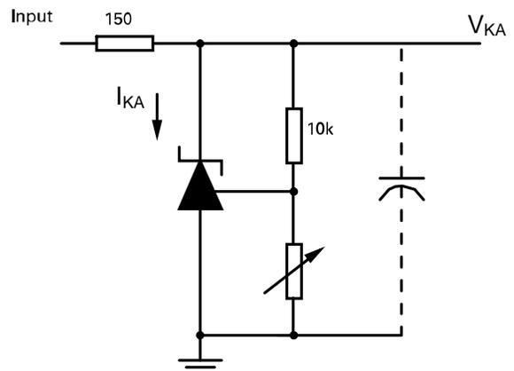
$V_{REF} < V_{KA} < 20$ ,  $I_{KA} = 10\text{mA}$ ,  $T_A = 25^\circ\text{C}$
