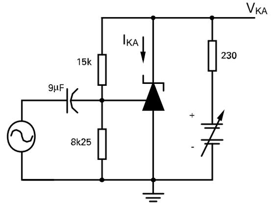
$I_{KA} = 10\text{mA}$ ,  $T_A = 25^\circ\text{C}$
