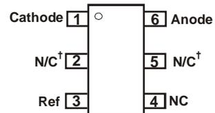
†Connected internally to substrate; should be left floating or connected to Anode
