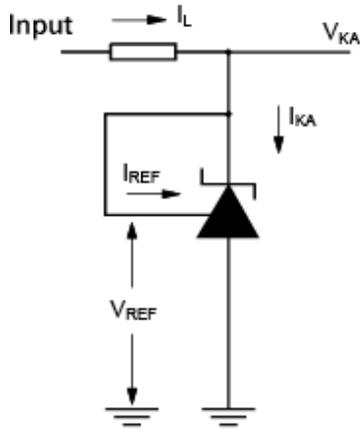
Figure 1. Test circuit for  $V_{KA} = V_{REF}$
