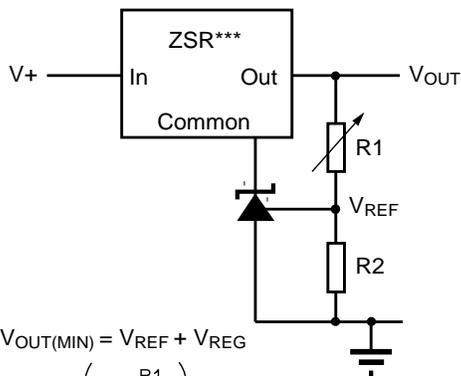
$$V_{OUT(MIN)} = V_{REF} + V_{REG}$$
