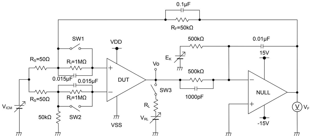
Figure 25. Test Circuit 1
