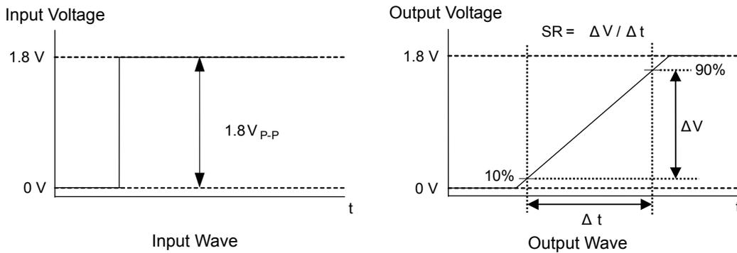
Figure 27. Slew Rate Input and Output Wave
