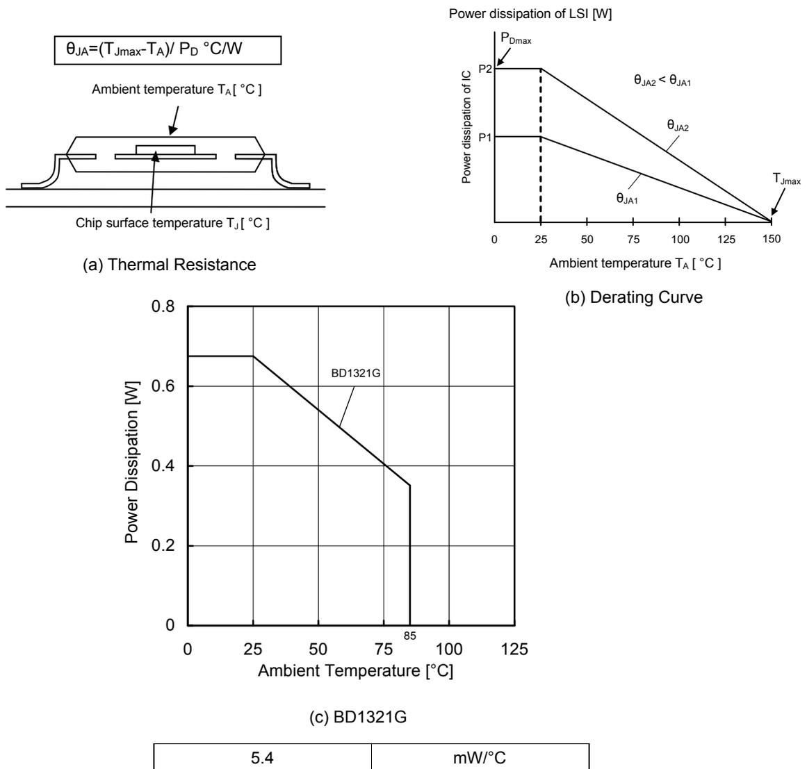
When using the unit above  $T_A=25^{\circ}\text{C}$ , subtract the value above per degree  $^{\circ}\text{C}$ . Permissible dissipation is the value when FR4 glass epoxy board 70mm  $\times$  70mm  $\times$  1.6mm (copper foil area below 3%) is mounted
