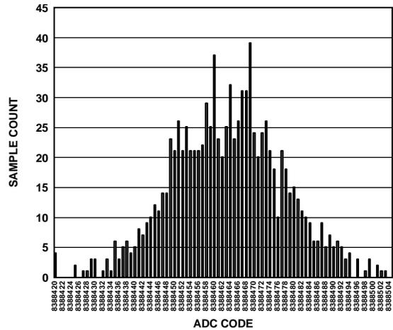
Figure 10. Histogram (Analog Input Buffers Disabled, V<sub>REF</sub> = 5 V, Output Data Rate = 250 kSPS)
