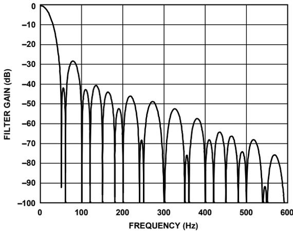
Figure 59. 27.27 SPS ODR, 36.67 ms Settling Time
