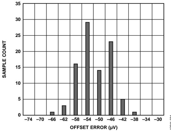
Figure 30. Offset Error Distribution Histogram (Internal Short, 92 Units)
