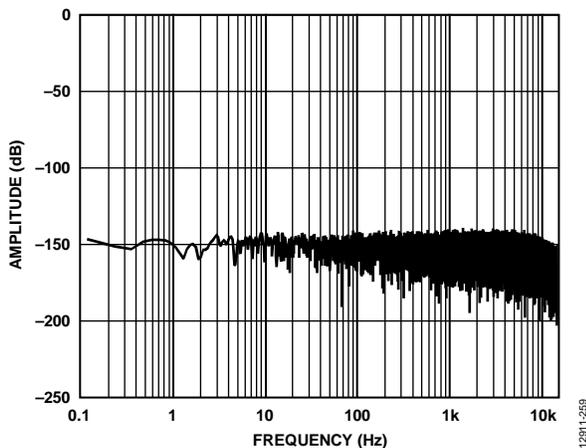
Figure 50. Shorted Input FFT (Analog Input Buffers Enabled)
