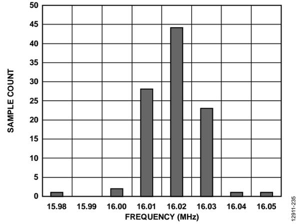
Figure 27. Internal Oscillator Frequency/Accuracy Distribution Histogram (100 Units)
