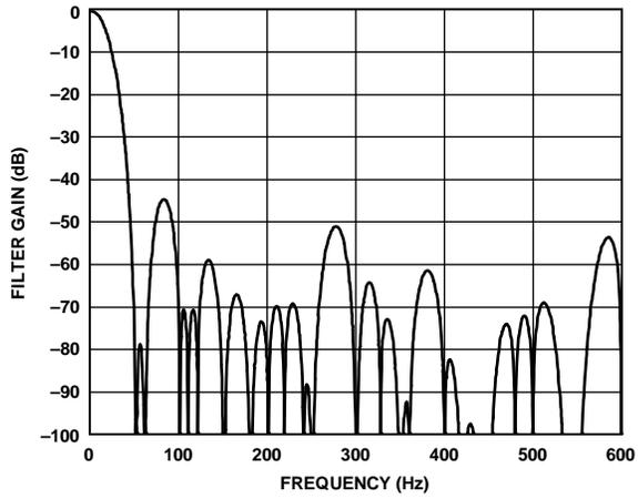
Figure 65. 16.667 SPS ODR, 60 ms Settling Time
