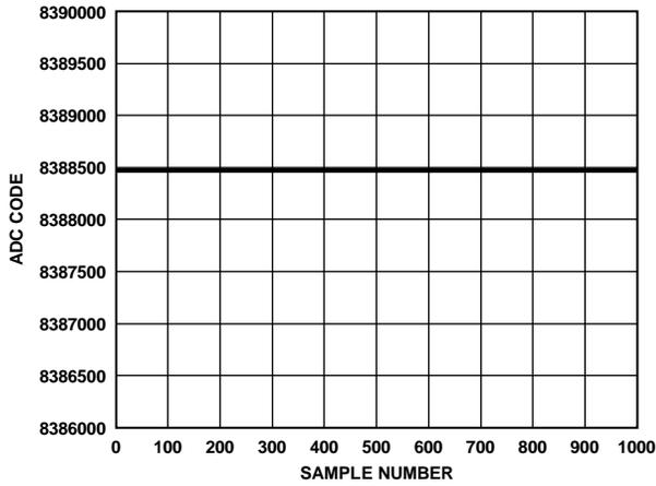
Figure 5. Noise (Analog Input Buffers Disabled, V<sub>REF</sub> = 5 V, Output Data Rate = 5 SPS)
