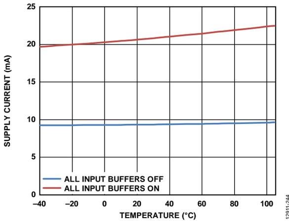
Figure 36. Supply Current vs. Temperature (Continuous Conversion Mode)
