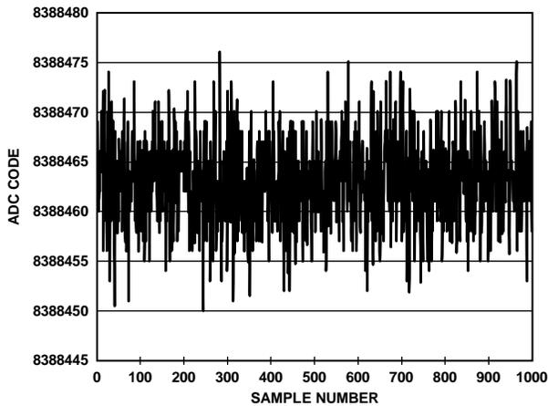
Figure 6. Noise (Analog Input Buffers Disabled, V<sub>REF</sub> = 5 V, Output Data Rate = 10 kSPS)
