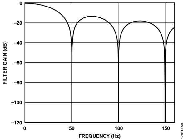
Figure 55. Sinc5 + Sinc1 Filter Response at 50 SPS ODR
