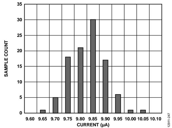
Figure 39. Burnout Current Distribution Histogram (100 Units)
