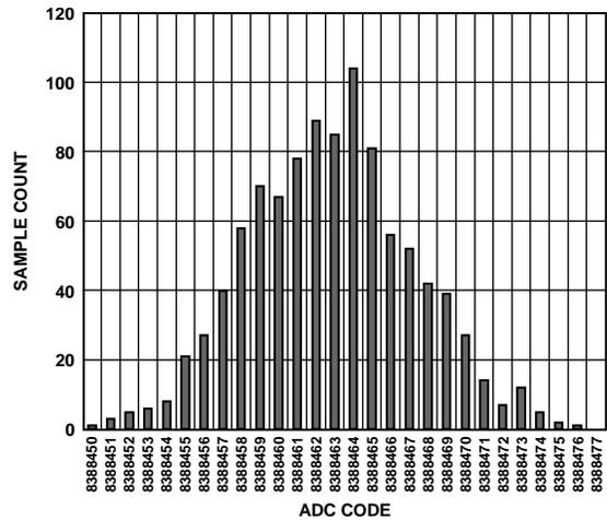
Figure 9. Histogram (Analog Input Buffers Disabled, V<sub>REF</sub> = 5 V, Output Data Rate = 10 kSPS)
