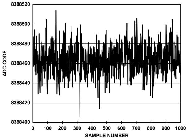
Figure 7. Noise (Analog Input Buffers Disabled, V<sub>REF</sub> = 5 V, Output Data Rate = 250 kSPS)
