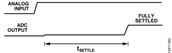
Figure 58. Step Input with Single Cycle Settling
