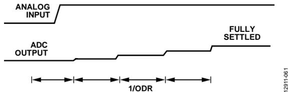
Figure 57. Step Input Without Single Cycle Settling
