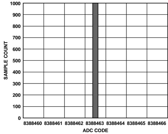
Figure 8. Histogram (Analog Input Buffers Disabled, V<sub>REF</sub> = 5 V, Output Data Rate = 5 SPS)
