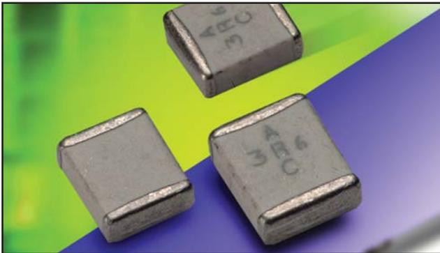
These porcelain and ceramic dielectric multilayer capacitor (MLC) chips are best suited for RF/ Microwave applications typically ranging from 10 MHz to 4.2 GHz. Characteristic is a fine grained, high density, high purity dielectric material impervious to moisture with heavy internal palladium electrodes.
