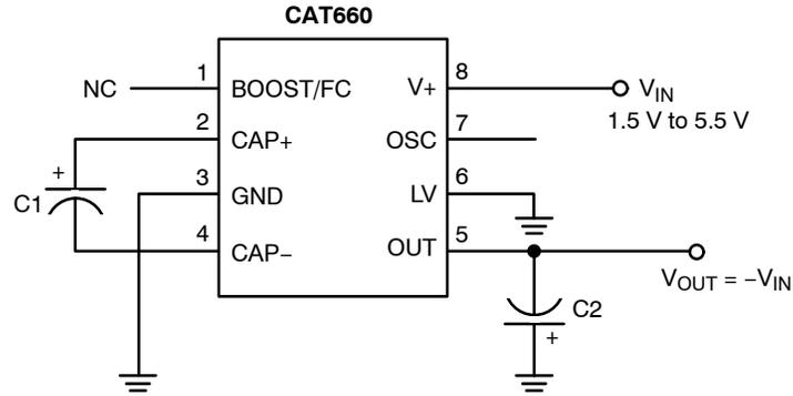
Figure 18. Voltage Inverter
