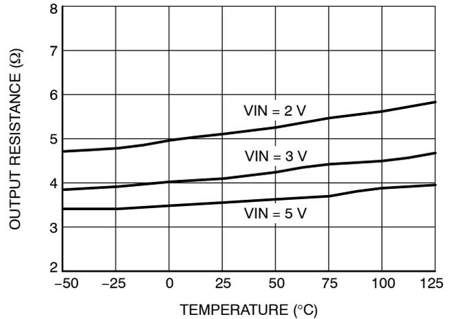
Figure 7. Output Resistance vs. Temperature (50 Ω Load)
