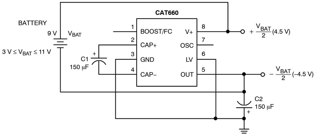
Figure 21. Battery Splitter
