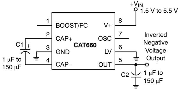
Figure 1. Voltage Inverter
