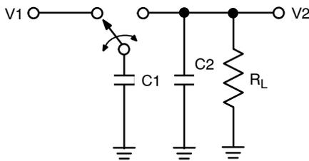
**Figure 13. Switched–Capacitor Building Block**
