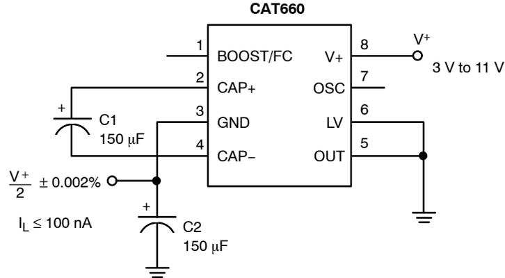
Figure 20. Precision Voltage Divider (Load  $\leq 100 \text{ nA}$ )
