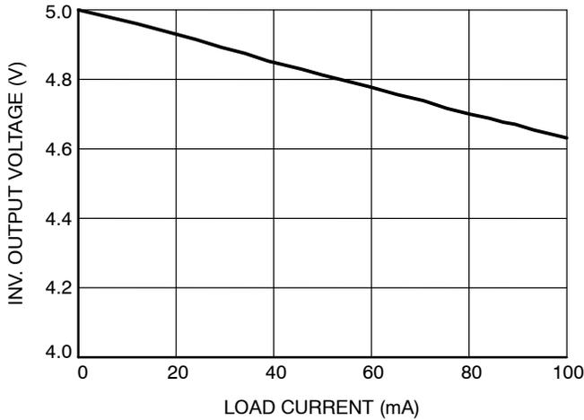
Figure 8. Inverted Output Voltage vs. Load, V+ = 5 V
