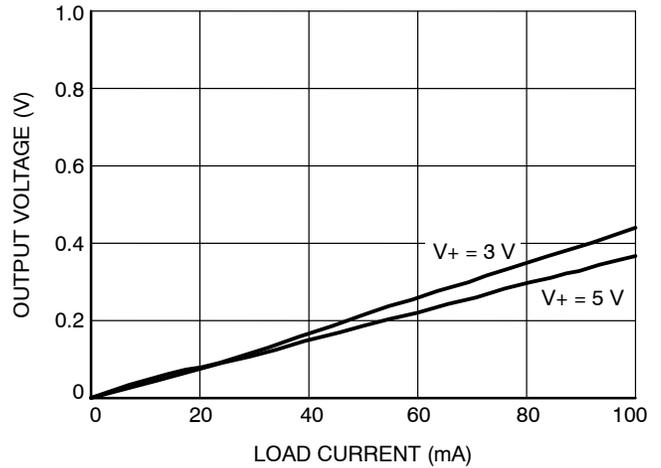
Figure 9. Output Voltage Drop vs. Load Current
