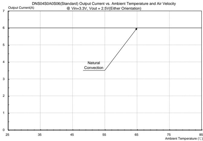
**Figure 48:** DNS04S0A0S06(Standard) Output current vs. ambient temperature and air velocity @Vin=3.3V, Vout=2.5V(Either Orientation)
