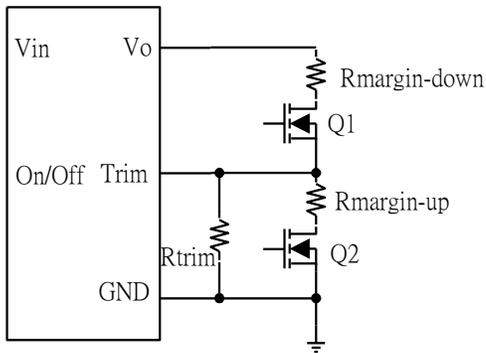
**Figure 39:** Circuit configuration for output voltage margining
