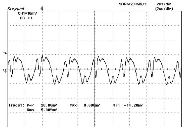
Figure 10: Output ripple & noise at 5Vin, 1.8V/6A out
