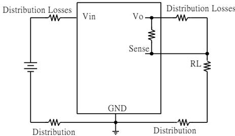
**Figure 36:** Effective circuit configuration for remote sense operation
