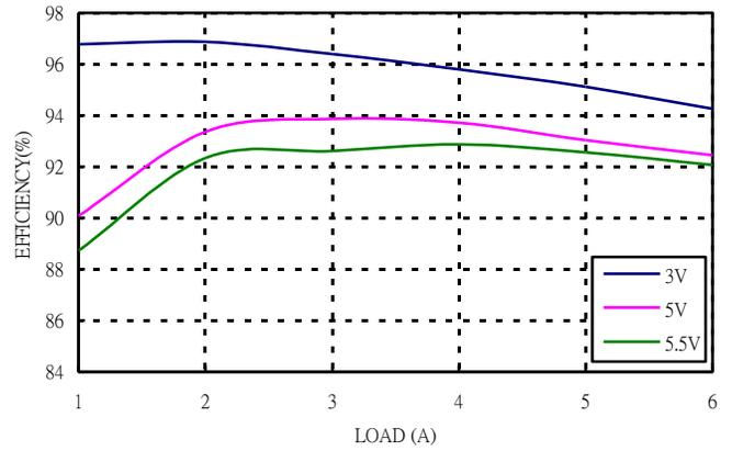
Figure 2: Converter efficiency vs. output current (2.5V out)
