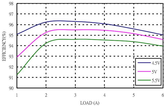
Figure 1: Converter efficiency vs. output current (3.3V out)
