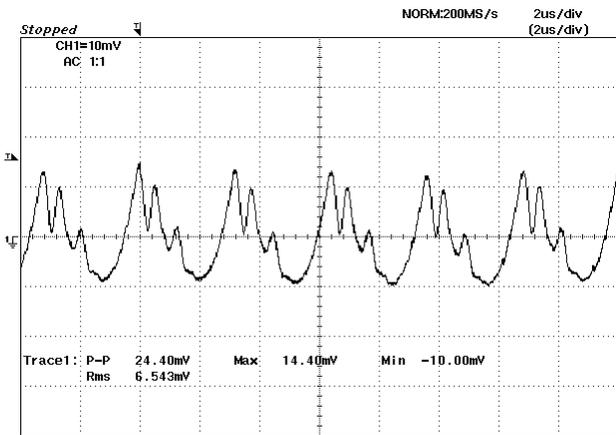
Figure 9: Output ripple & noise at 5Vin, 3.3V/6A out
