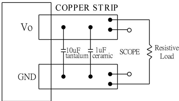
Note: Use a 10µF tantalum and 1µF capacitor. Scope measurement should be made using a BNC connector.
