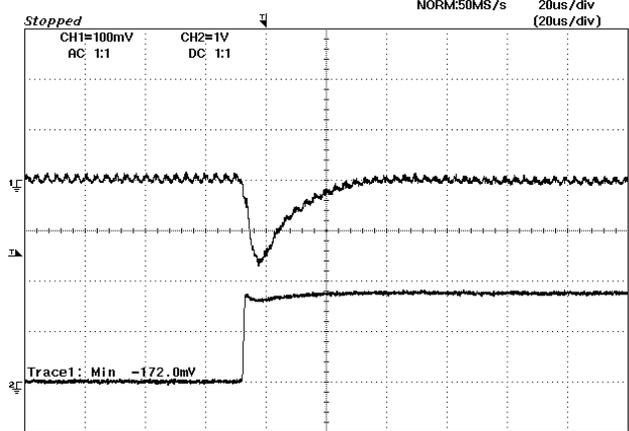
**Figure 25:** Typical transient response to step load change at  $2.5A/\mu S$  from 100% to 50% of  $I_o$ , max at 3.3Vin, 1.8Vout ( $C_{out} = 1\mu F$  ceramic,  $10\mu F$  tantalum)
