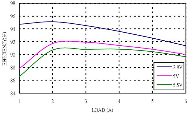
Figure 3: Converter efficiency vs. output current (1.8V out)
