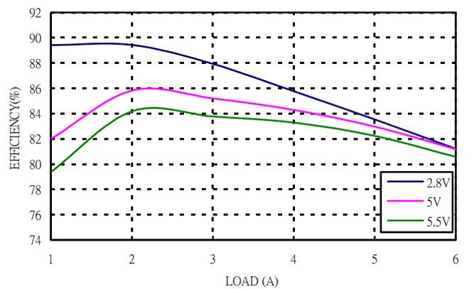
Figure 6: Converter efficiency vs. output current (0.75V out)
