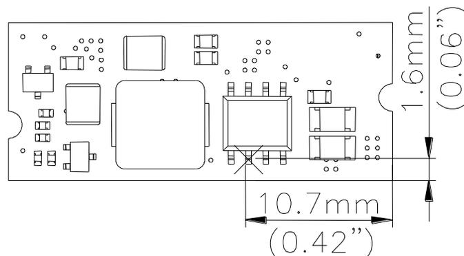
**Figure 44:** Temperature measurement location
