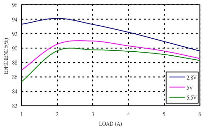
Figure 4: Converter efficiency vs. output current (1.5V out)
