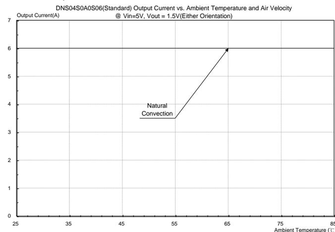
**Figure 46:** DNS04S0A0S06(Standard) Output current vs. ambient temperature and air velocity @ Vin=5V, Vout=1.5V(Either Orientation)
