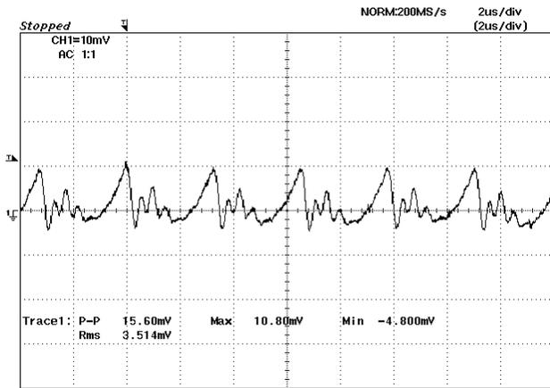
Figure 7: Output ripple & noise at 3.3Vin, 2.5V/6A out
