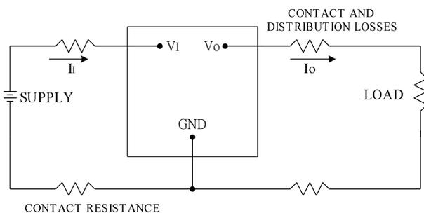
**Figure 31:** Output voltage and efficiency measurement test setup
