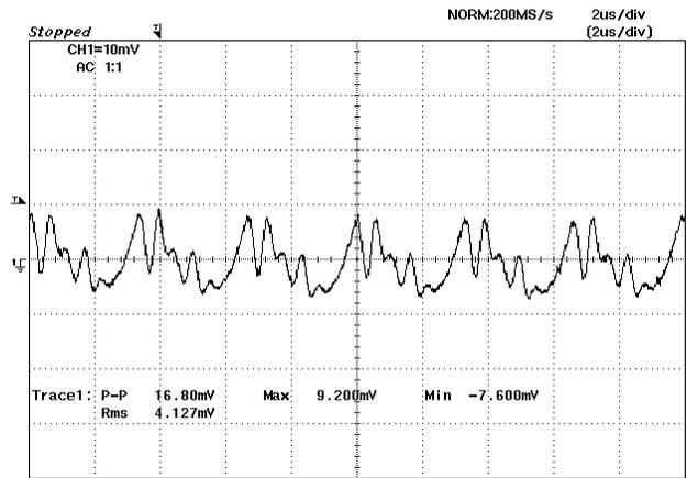
Figure 8: Output ripple & noise at 3.3Vin, 1.8V/6A out
