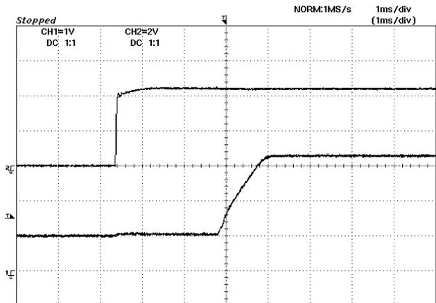
**Figure 27:** Output short circuit current 5Vin, 0.75Vout
