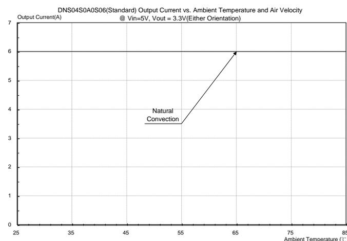
**Figure 45:** DNS04S0A0S06(Standard) Output current vs. ambient temperature and air velocity @ Vin=5V, Vout=3.3V(Either Orientation)
