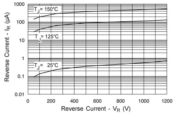
Fig. 2 - Typical Reverse Current vs. Reverse Voltage
